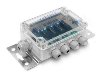
IP67 junction box fitted with electronic board for junction and equalisation of 2, 3, or 4 load cells. Terminal boards with a screw for easing the connection of the load cells and the signal adjustment trimmer, for an accurate and reliable equalisation.
